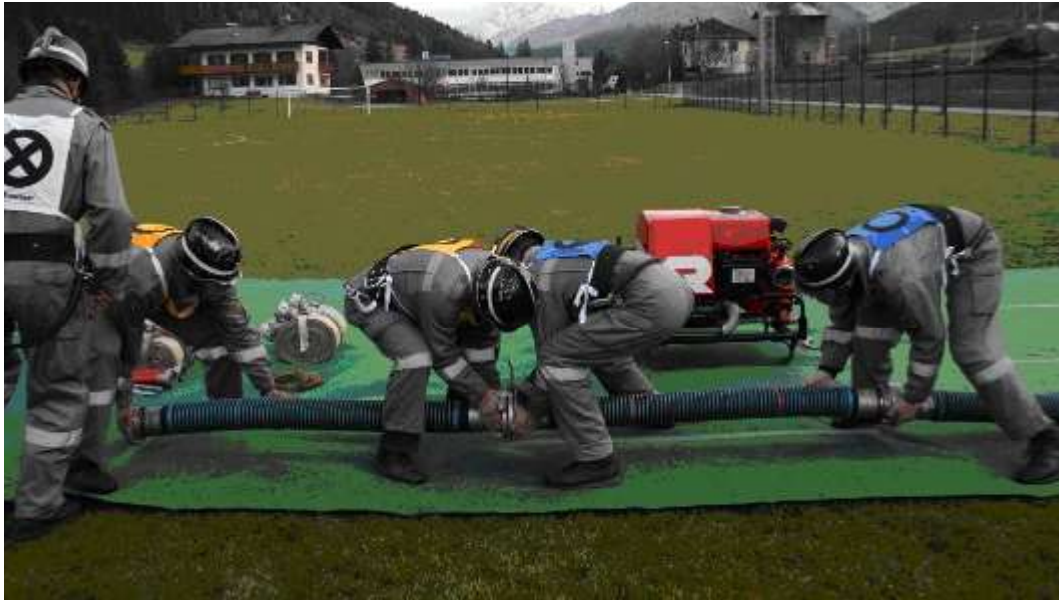
Fig. 17: Pump operator supervises the coupling of the suction pipe by the water troop and hose troop
