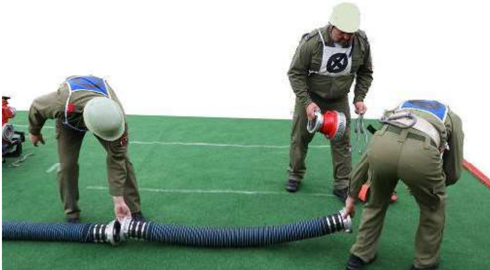
Fig.9: The correctly laid out suction hoses - the suction head is handed over
