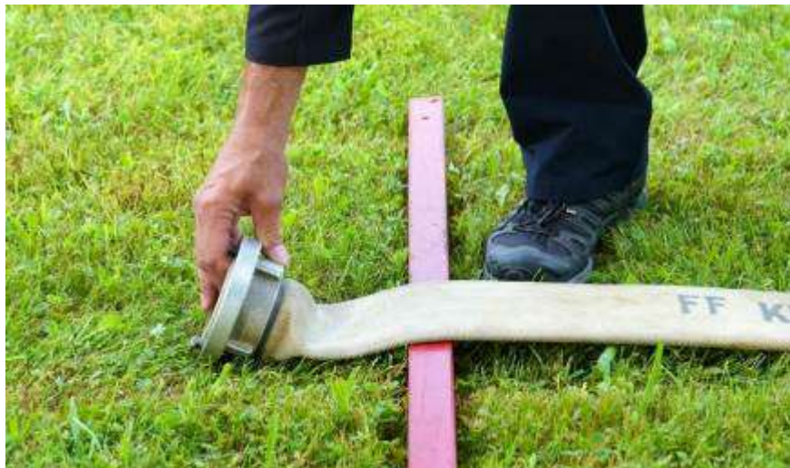
Fig.28a: Correct position of the coupling of the second B-hose
