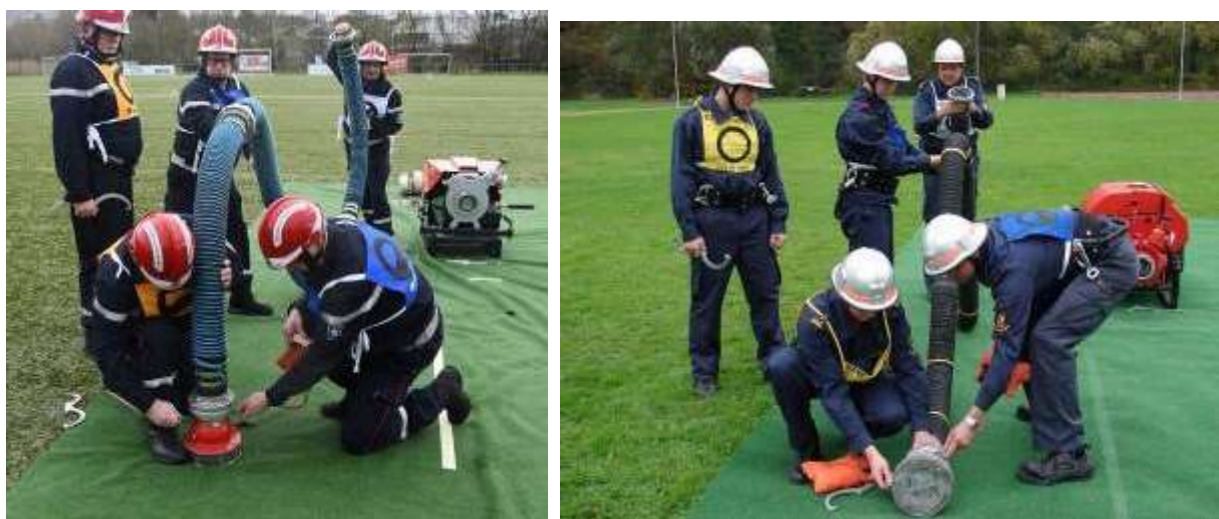
Fig.21/fig.21a: Lifting of the coupled suction hose rope, attaching of the suction hose and valve rope
