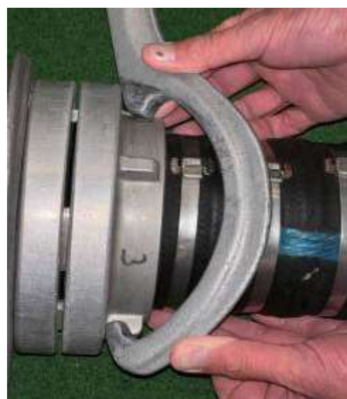
Fig. 18: Attaching the coupling keys and coupling of the suction hoses
