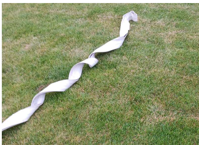
Fig.33a: badly laid-out pressure hose
