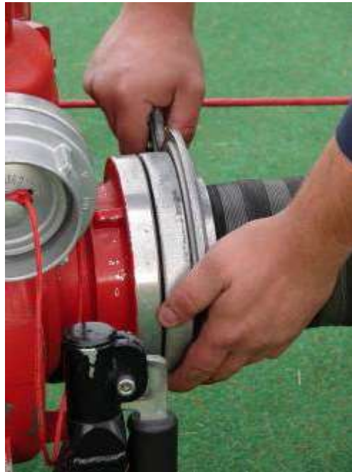
Fig.24a: Placed coupling key - no "knocking", otherwise "faulty work"
